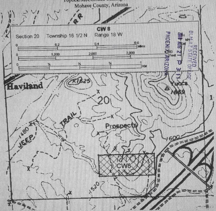
The Claim is delineated thusly: From the NW corner, 600 feet at approximately 180° to the SW corner, then 1500 feet at approximately 90° to the SE Corner, then 600 feet at approximately 0° to the NE corner, then 1500 feet at approximately 270° to the point of beginning.
